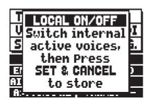
To set a voice in Local Off mode, operate its draw-stop or rocker switch so that its light goes out. After setting the setup required, press [S] and [C] together to save it.
