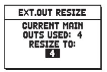
The **CURRENT MAIN OUTS USED** parameter points out the amount of outputs currently used by the External Routers, as set in the EXTERNAL OUT ROUTER function.
