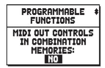
To switch off the light of MIDI stops and [M.SOLO] pistons, when the Cancel piston is pressed (this screen is available only in models that allow to transmit MIDI codes).
