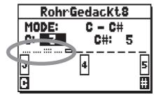
Pressing [ENTER] from the previously described message confirms the current routing, the overlapping voices will not be audible except with the sub-woofer(s) and it is recommended to check and/or modify the assignment on the MAIN outputs.
