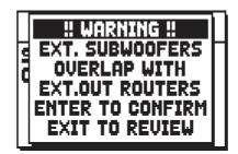
informs that one or more voice outputs have been addressed to MAIN outputs already configured for use with sub-woofer (see section 9.9). These outputs are also shown on the display area in the screen showing the total outputs. If two dot lines are displayed, this indicates that one or more overlaps are present:
