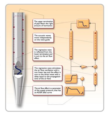
incorporating the principal physical parameters ie. construction geometry, materials used, and pertaining air pressure, etc.
