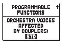
in models equipped with sub- and super-octave couplers, and/or with unison off couplers, the user can select which of these couplers will affect the orchestra stops:
