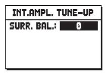
Set the SURR. BAL. (surround balance) parameter as 0 to distribute the signal evenly on both sides. The other parameters are accompanied by an arrow: from \(\xi\) 1 to \(\xi\) 63 the signal is diffused more and more to the left, while values from \(\xi\) 1 to \(\xi\) 63 send more signal to the right speakers.
