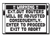
The system will warn you that the external panning of the stops will be modified automatically (according to the outputs in use). Press [EXIT] to abort and go back to the SET-UP menu. Press [ENTER] to continue: the following screen will show:
