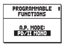
Select PD/II MONO or PD/I MONO to activate the Monophonic Pedal function (with piston on). This function allows to play pedalboard registers on Manual II (in three nad four-manual models) or on Manual I (in two-manual models). When doing this the pedalboard is deactivated and the stops become monophonic, with priority on the lowest note.
