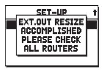
The repositioning takes place through several adjustments, so as to use the outputs as already configured before. However, some routers might be placed differently from what you intended. Therefore, at the end of the procedure, the system will advice to check again the settings through the EXTERNAL OUT ROUTER function.
