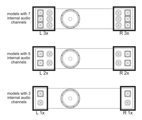
Arranging the voices in the two channels simulates the position of the windchests of real pipe organs, since they were usually placed in different areas. It also simulates the different position of the pipes inside the windchest, which could vary according to the stop played, the period when the organ was built and the wishes of the builder.
