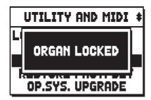
To unlock the organ, allow the saving of combinations and make the other adjustment functions accessible, recall the UNLOCK ORGAN function under the UTILITY & MIDI menu (see next page).
