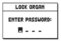
Press [VALUE +] and [VALUE -] to select the characters. Use the [FIELD  $\blacktriangle$ ] and [FIELD  $\blacktriangledown$ ] buttons to move the cursor. Press [ENTER] to save the code, and [EXIT] to abort.
