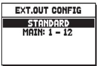
Use the [VALUE +] and [VALUE -] buttons to select the desired configuration. Then press ENTER] to confirm the selection or [EXIT] to cancel. After selecting a new configuration, the following warning pop-up is displayed:
