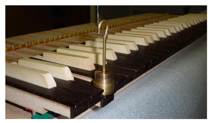
Testing and verify that the key stays on rest position with 120g of weight.
