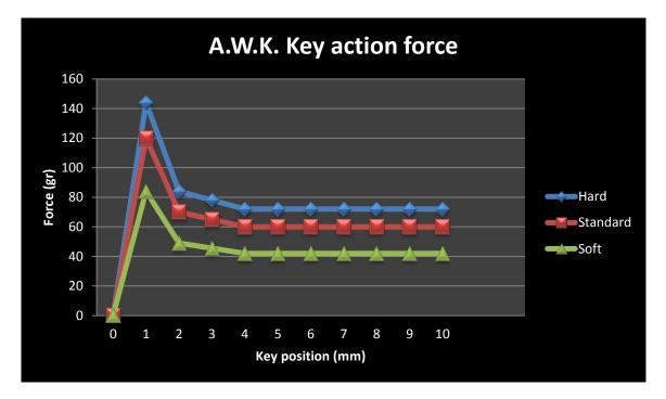
The A.W.K. key action force reproduce the typical behavior of real pipe organ keyboard with mechanical transmission.
