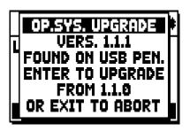
In this phase the system checks the upgrade installation files in your flash drive. As written on the pop-up, press [ENTER] to proceed, or [EXIT] to abort.
