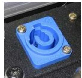
Powercon connectors (a female connector is shown in the figure on the right) is used to provide AC current to the speakers in chain from a single power source. Never exceed maximum current limits for devices, equipment, cables, etc. The mains cable provided with your OUTSIDER318 can supply up to 16A, hence it is possible to cascade up to 3 loudspeakers (including the one connected to the mains).
