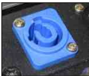
Detail of a Powercon main input
